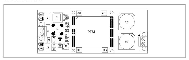
Figure 19 — The PFM evaluation board shown (actual size) above illustrates the layout and compact size of a complete AC to 48 Vdc, 200 Watt front end power supply using the PFM.
