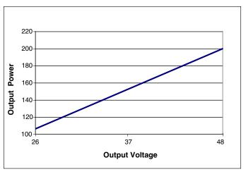
Figure 7 — Output power rating vs. trimmed output voltage
