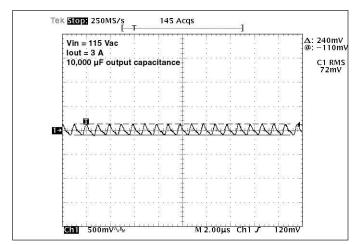
Figure 16 — Output Ripple (Switching frequency)
