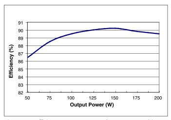
Figure 9 — Efficiency vs. Output Power (120 Vrms, 48 Vdc)
