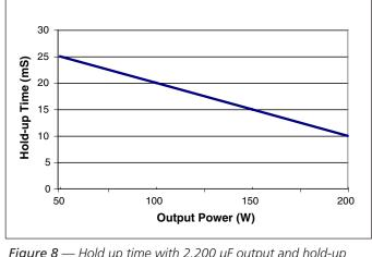
Figure 8 — Hold up time with 2,200 μF output and hold-up capacitors with 48 Vdc output
