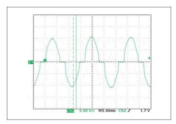
Figure 13 — Typical Input Current (230 Vrms 200 W Out)
