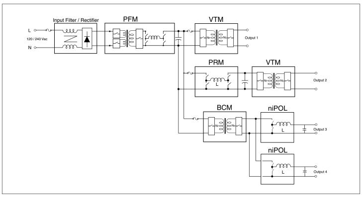
Figure 20 — Typical application using Factorized Power Architecture (FPA)
