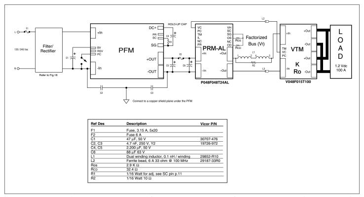
Figure 17 — Typical FPA (Factorized Power Architecture) from the wall plug to the point of load. See PRM data sheet (P048F048T24AL) for other output voltage / current options.
