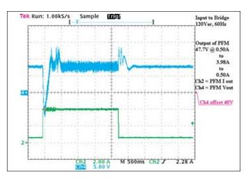
Figure 14 — Transient Response Input:120 Vac, 60 Hz Output step load: 10% to 90% to 10%
