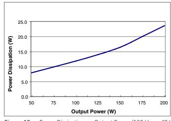
Figure 10 — Power Dissipation vs. Output Power (120 Vrms, 48 Vdc)
