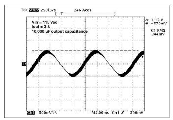
Figure 15 — Output Ripple (Line frequency)
