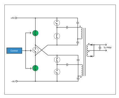
Figure 3— 120 Vac input configuration
