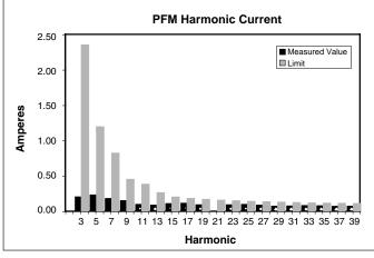
Figure 11 — Harmonic Current vs. EN61000-3-2 limits (115 Vrms 180 W Out)
