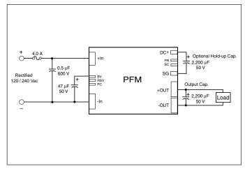
Figure 12 — PFM test circuit
