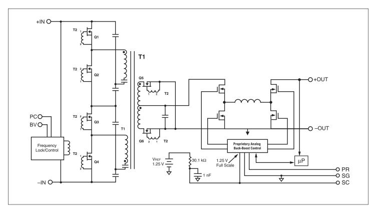
Figure 6 — Functional block diagram of the PFM
