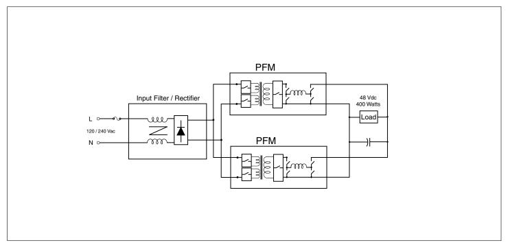
Figure 21 — Two PFMs operated in parallel for additional power.
