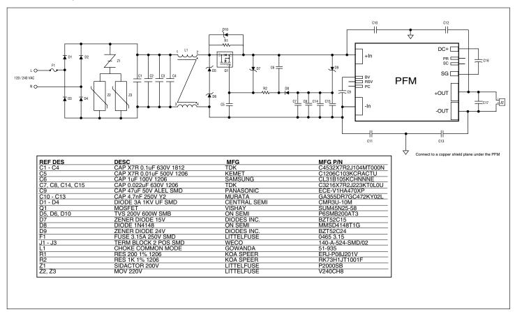
Figure 18 — Typical application circuit
