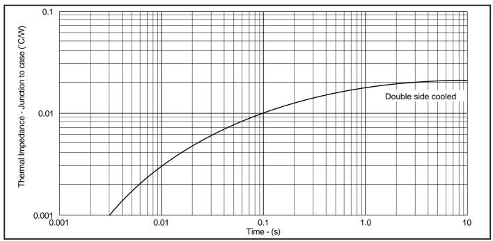
Fig.3 Maximum (limit) transient thermal impedance - junction to case - (°C/W)
