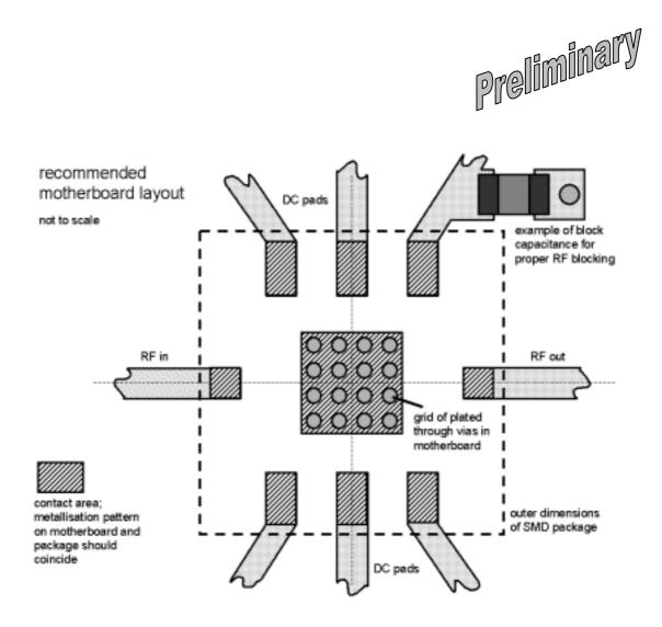
The RF ports comprise a DC blocking capacitor on chip level. The DC connections include a first level of DC decoupling capacitors (typically 120pF) in the package. However, all DC bias ports should be additionally connected to ground with 10nF capacitors at board level to prevent the MMIC from oscillations. These parts should be placed close to the SMD leadless package. If the same bias is required at different DC ports, the lines should only be connected behind these block capacitors.
