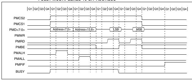
FIGURE 11-26: WRITE TIMING, 16-BIT MULTIPLEXED DATA, FULLY MULTIPLEXED 16-BIT ADDRESS
