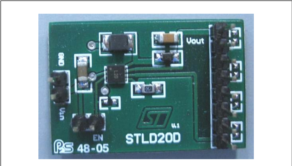
Figure 25. Evaluation board top view with its connections at the external equipment
