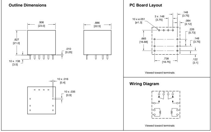
Dimensions in inches with metric equivalents in parentheses. Tolerance: ± 0.010"
