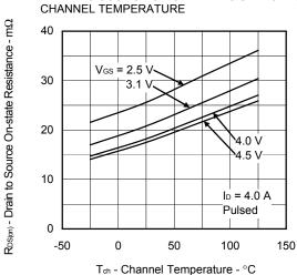
DRAIN TO SOURCE ON-STATE RESISTANCE vs.
