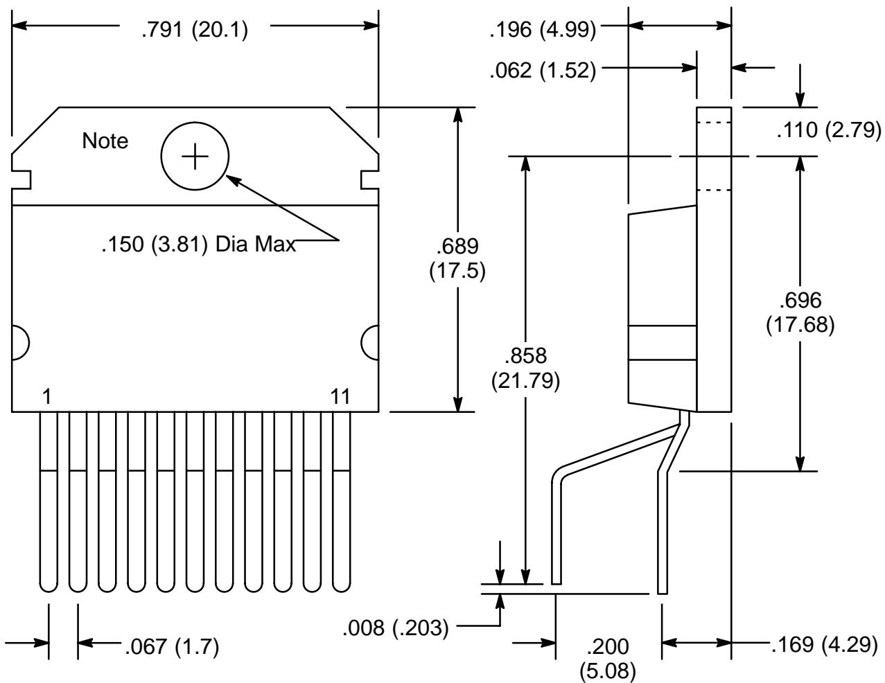
**NOTE:** Tab connected to Pin 6
