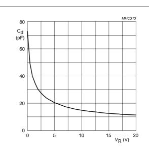
Schottky barrier diode; f = 1 MHz;  $T_{amb}$  = 25 °C.
