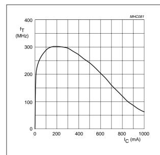
NPN transistor;  $V_{CE} = 10 \text{ V}.$
