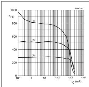
NPN transistor;  $V_{CE} = 5 \text{ V}$ .
