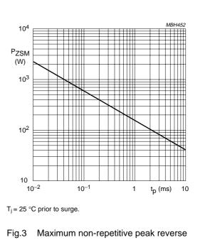
Fig.3 Maximum non-repetitive peak reverse power dissipation as a function of pulse duration (square pulse).
