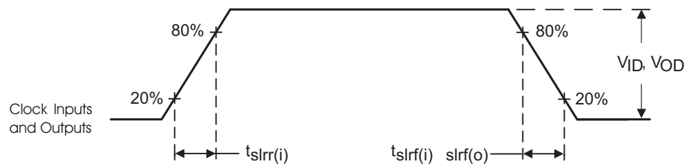
Figure 8. Input and Output Slew Rates
