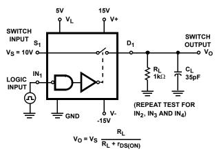
FIGURE 2. SWITCHING TIME TEST CIRCUIT
