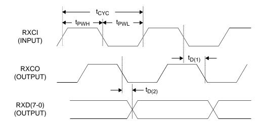
Note: Shown for RINVC equal to 0. Data is clocked out on positive transitions when control bit RINVC is equal to 1.
