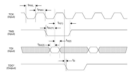
\*Note: TDO is a three-state output. If this pin is used, it should be connected via a 4.7 k $\Omega$  resistor to the +5 volt supply.
