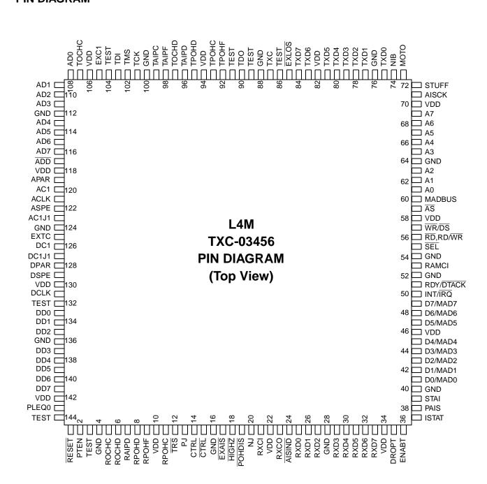
Figure 2. L4M TXC-03456 Pin Diagram
