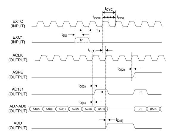
Figure 6. Add Bus Interface Timing (External Clock)
