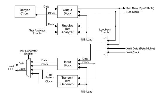
Figure 23. Test Generator, Analyzer and Loopback
