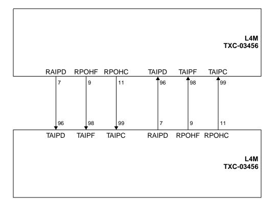
Figure 27. Use of Two L4M Devices in Ring Configuration
