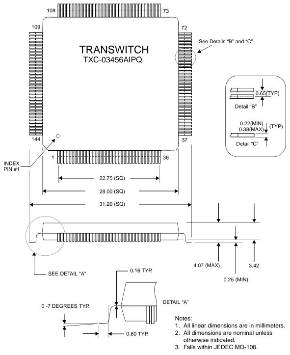
Figure 28. L4M TXC-03456 144-Pin Plastic Quad Flat Package
