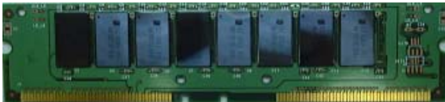
Note: On double sided modules, RDRAM devices are also installed on bottom side of PCB.
