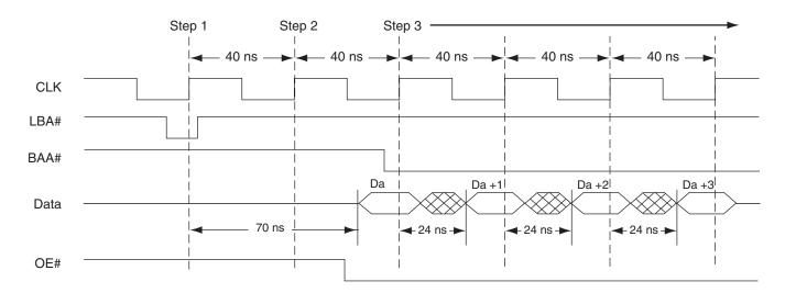
Figure 4. Burst Mode Read with 25 MHz CLK, 70 ns t<sub>IACC</sub>, 24 ns t<sub>BACC</sub> Parameters
