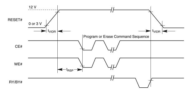
Figure 23. Temporary Sector Unprotect Timing Diagram
