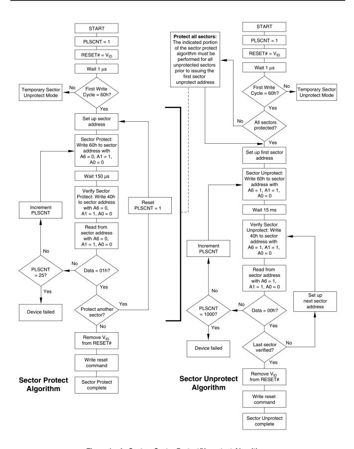
Figure 1. In-System Sector Protect/Unprotect Algorithms
