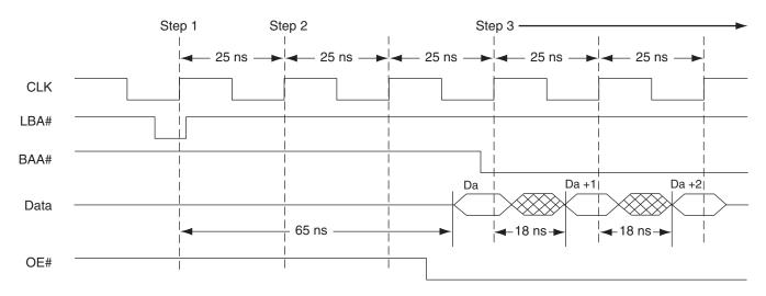
Figure 3. Burst Mode Read with 40 MHz CLK, 65 ns t<sub>IACC</sub>, 18 ns t<sub>BACC</sub> Parameters
