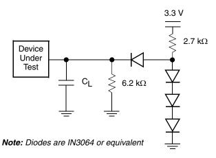
Figure 13. Test Setup
