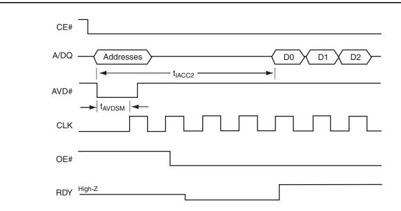
**Note:** If  $t_{AVDSM} > 1$  CLK cycle, wait state usage is reduced. Figure shows 40 MHz clock, handshaking enabled. Wait state usage is 4 clock cycles instead of 5. Note that  $t_{AVDSM}$  must be less than 76 µs for burst operation to begin.
