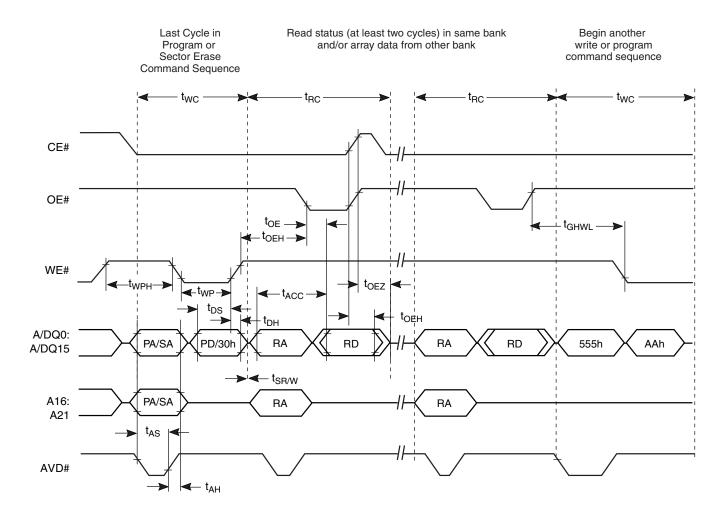
**Note:** Breakpoints in waveforms indicate that system may alternately read array data from the "non-busy bank" while checking the status of the program or erase operation in the "busy" bank. The system should read status twice to ensure valid information.
