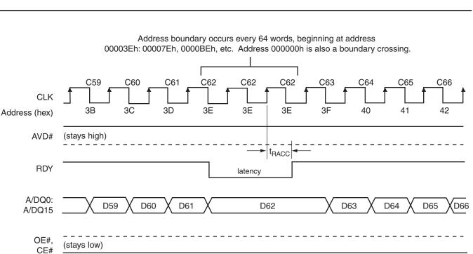
Figure 18. 8-, 16-, and 32-Word Linear Burst Address Wrap Around
