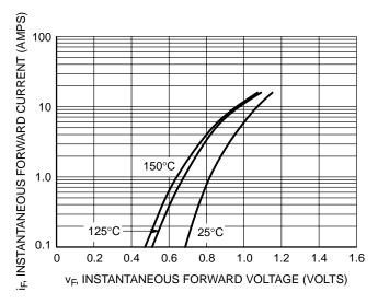
Figure 1. Typical Forward Voltage
