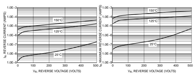
**Figure 3. Typical Reverse Current**
