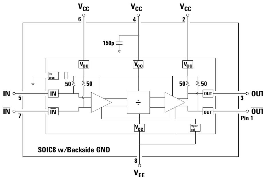
Figure 1. Simplified Schematic
