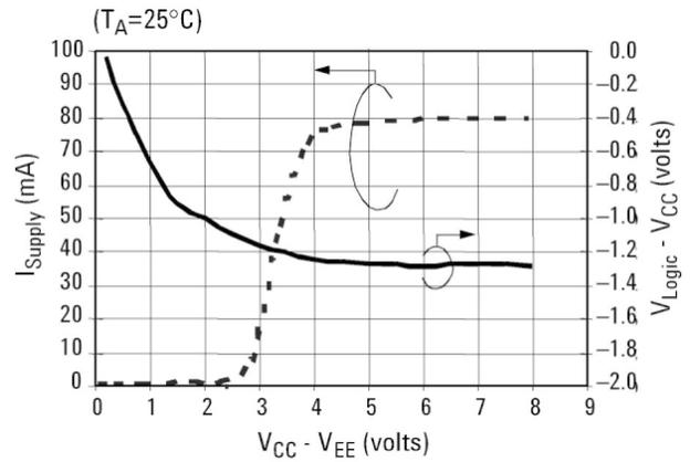
Figure 5. Typical Supply Current &  $V_{Logic}$  vs. Supply Voltage
