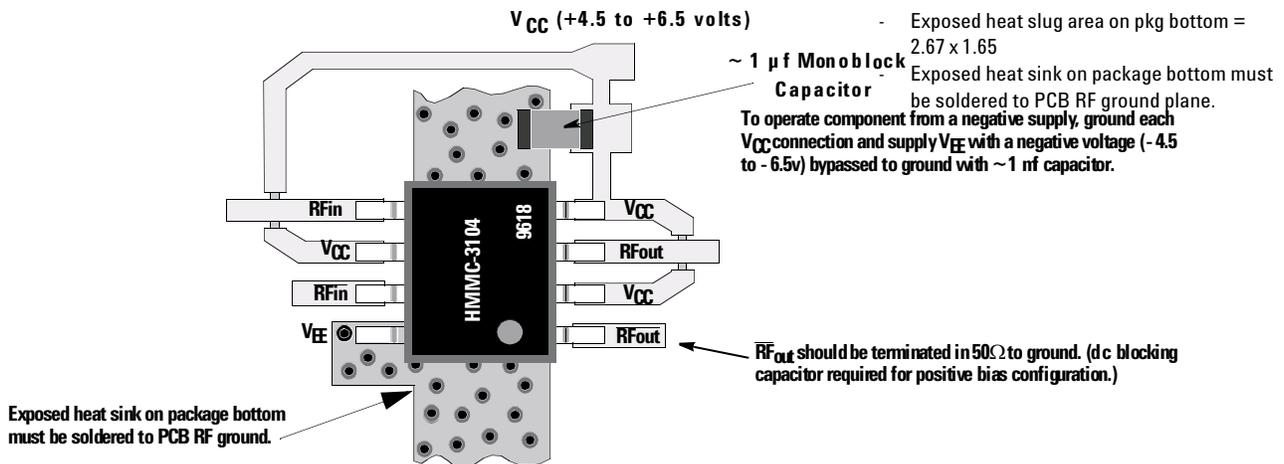
Figure 3. Assembly Diagram (Single-supply, Positive-bias Configuration shown)
