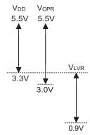
Note:  $V_{OPR}$  is the voltage range for proper chip operation at 4MHz system clock.
