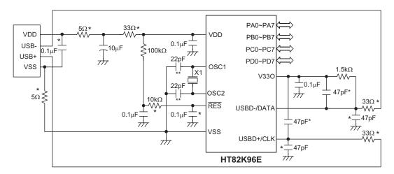
Note: The resistance and capacitance for reset circuit should be designed in such a way as to ensure that the VDD is stable and remains within a valid operating voltage range before bringing RES to high.
