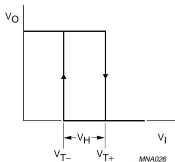
Fig.5 Transfer characteristic.
