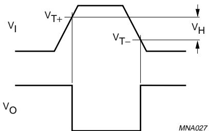
$V_{T+}$  and  $V_{T-}$  are between limits of 20% and 70%.Fig.6 The definitions of  $V_{T+}$ ,  $V_{T-}$  and  $V_H$ .
