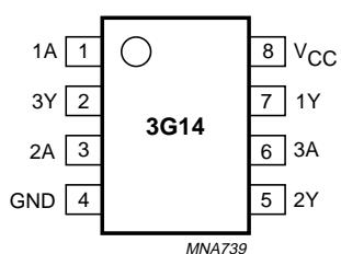
Fig.1 Pin configuration.
