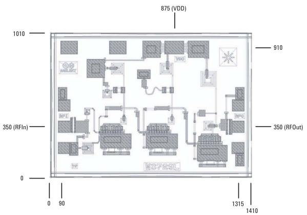
Figure 20. AMMC-5620 Bond Pad Locations.
