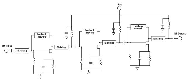
Figure 18. AMMC-5620 Schematic
