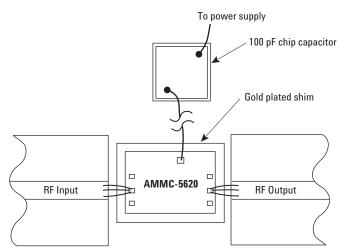
Figure 19. AMMC-5620 Assembly Diagram
