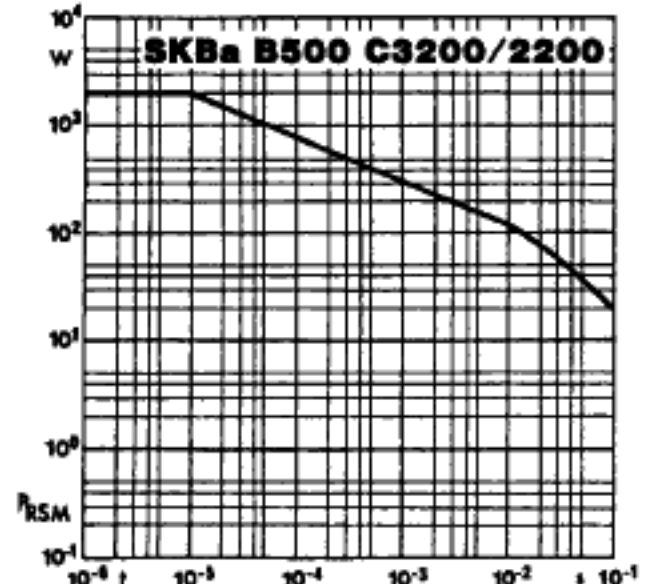
Fig. 7 Rated reverse power dissipation vs. time
