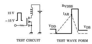
$\begin{array}{ll} \text{Peak IAR} = 5 \text{ A, RG} = 25 \, \Omega \\ \text{V}_{DD} = 25 \, \text{V, L} = 7 \, \text{mH} \end{array} \quad \text{E}_{AS} = \frac{1}{2} \cdot \text{L} \cdot \text{I}^2 \cdot (\frac{\text{BVDSS}}{\text{BVDSS} - \text{VDD}})$
