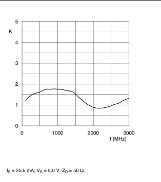
Fig.10 Stability factor as a function of frequency; typical values.
