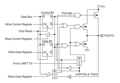
PC0/TX Input/Output Ports
