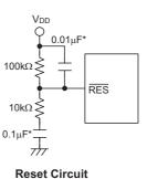
Note: "\*" Make the length of the wiring, which is connected to the RES pin as short as possible, to avoid noise interference.
