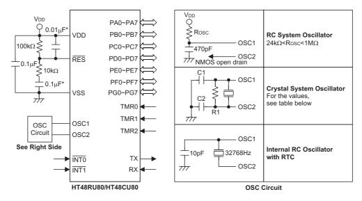
Note: The resistance and capacitance for reset circuit should be designed to ensure that the VDD is stable and remains in a valid range of the operating voltage before bringing RES high.
