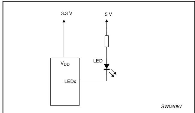
Figure 15. Device supplied by a lower voltage
