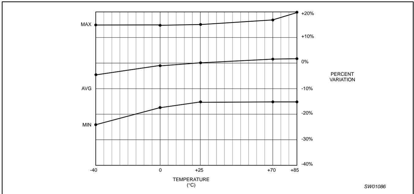
Figure 17. Typical frequency variation over process at V<sub>DD</sub> = 3.0 V to 5.5 V
