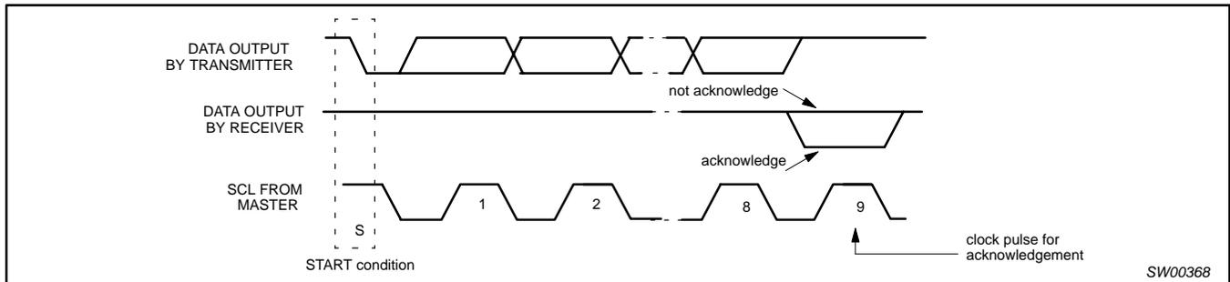
Figure 9. Acknowledgement on the I<sup>2</sup>C-bus
