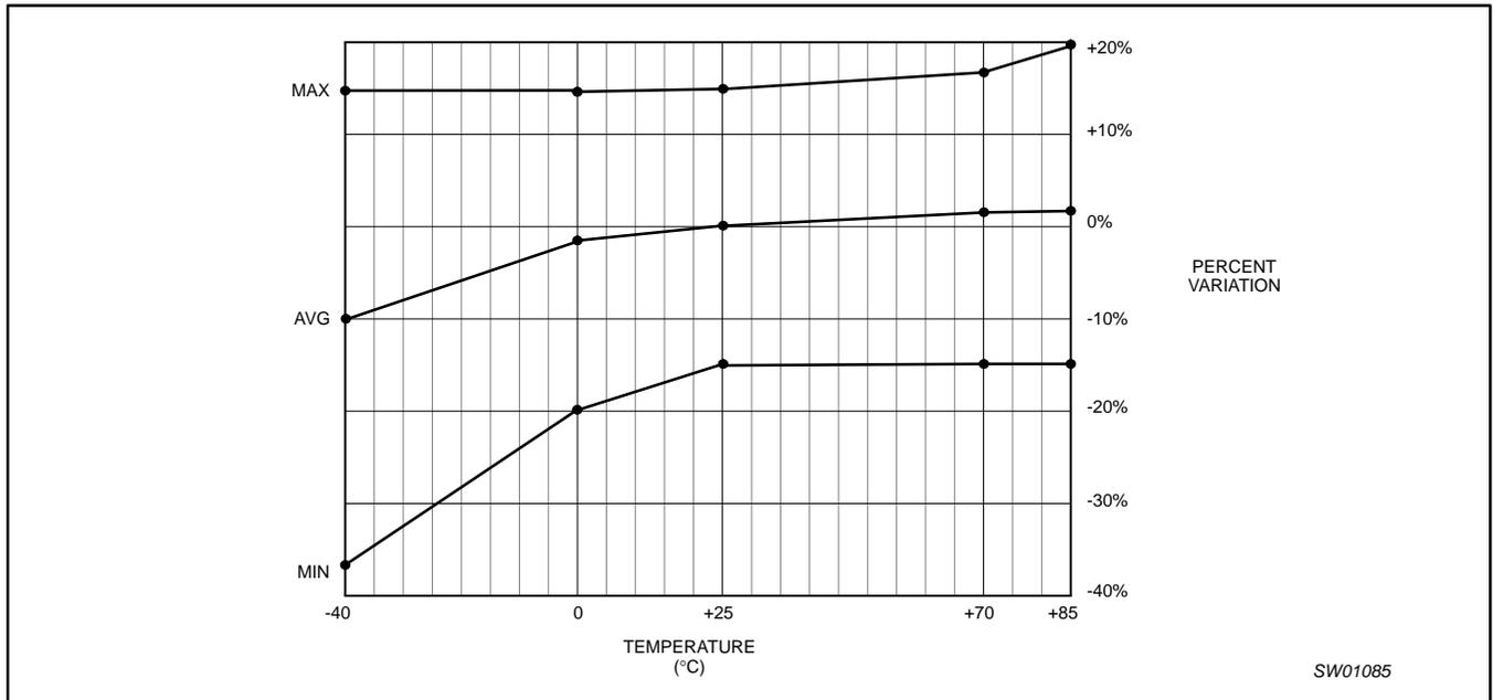
Figure 16. Typical frequency variation over process at V<sub>DD</sub> = 2.3 V to 3.0 V
