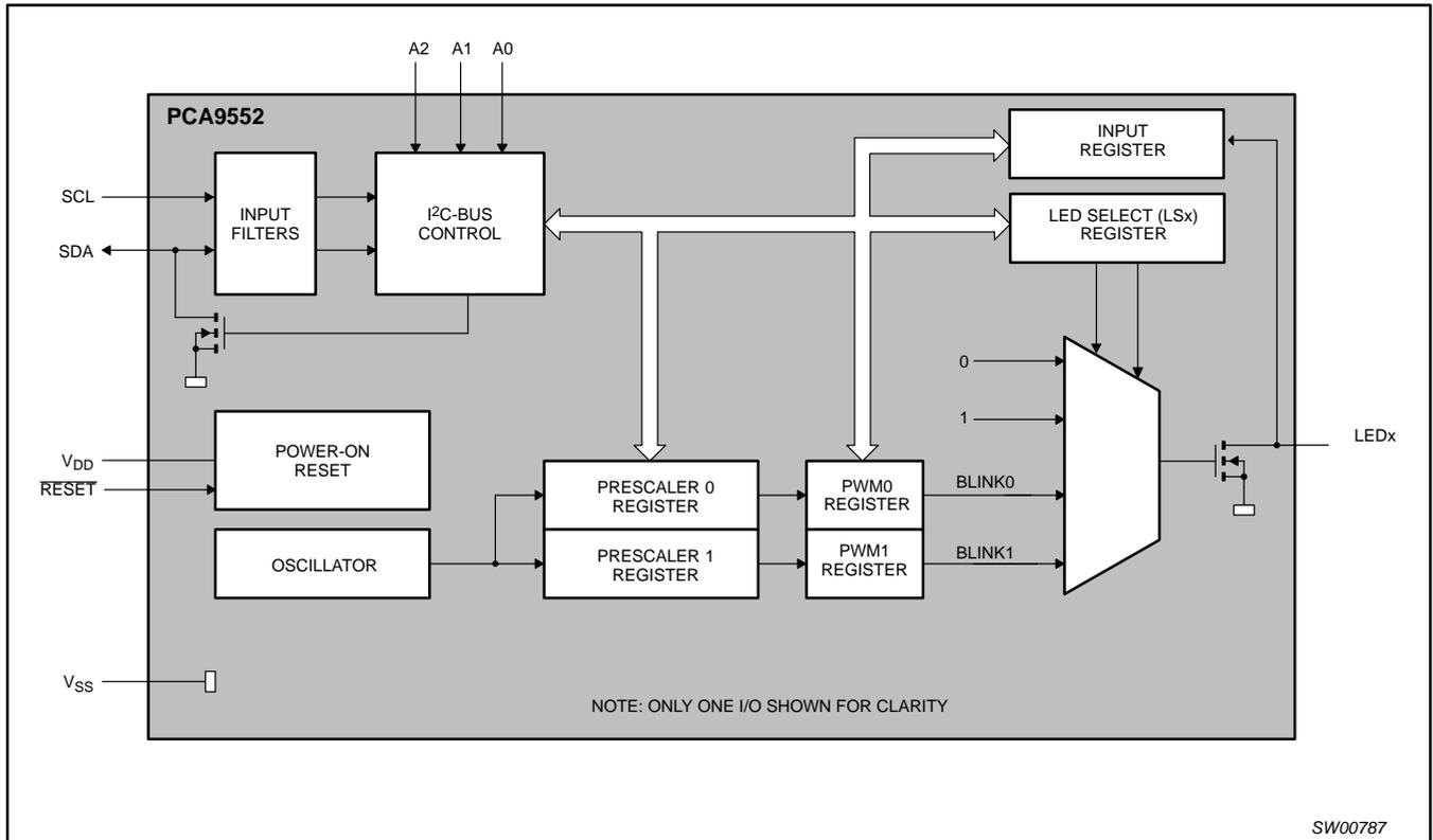
Figure 3. Block diagram
