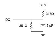
Fig. 2 OUTPUT LOAD EQUIVALENT
