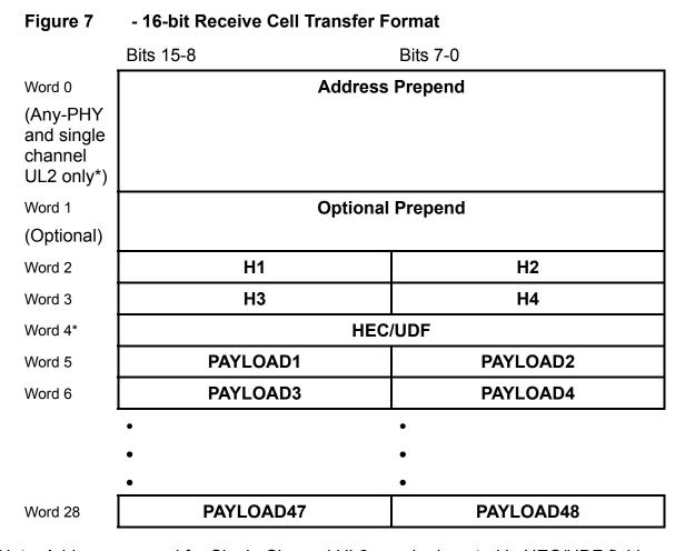
Note: Address prepend for Single Channel UL2 may be inserted in HEC/UDF field instead of prior to the cell.
