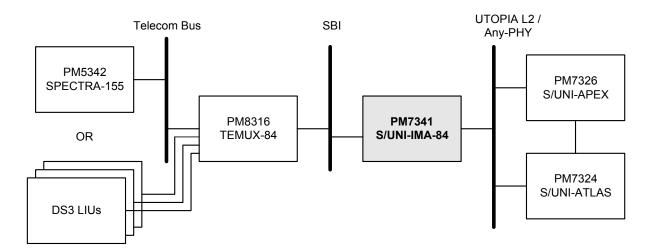
With a PM5313 SPECTRA-622, four TEMUX-84s, four S/UNI-IMA-84s, PM7326 S/UNI-APEX, and PM7324 S/UNI-ATLAS devices, an OC-12's worth of IMA/UNI circuits can be terminated on a single linecard.
