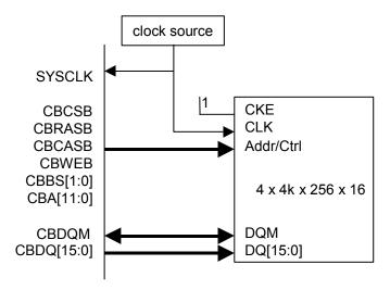
There are three processes, all of which are arbitrated by the SDRAM arbiter, that access the cell buffer SDRAM:
