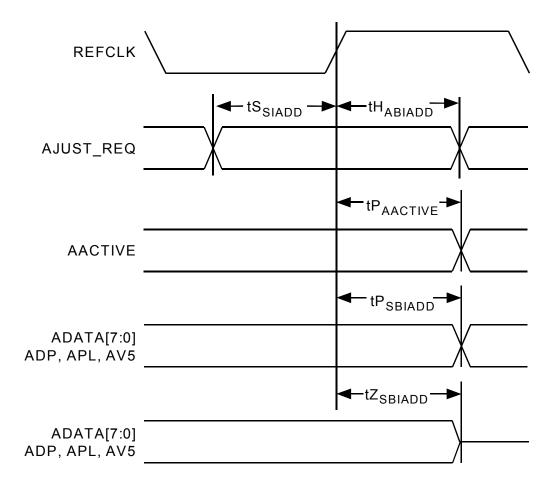
Figure 53 - SBI ADD BUS Collision Avoidance Timing
