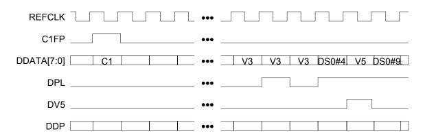
Figure 26 illustrates the operation of the SBI DROP Bus, using a negative justification on the second to last V3 octet as an example. The justification is indicated by asserting DPL high during the V3 octet. The timing diagram also shows the location of one of the tributaries by asserting DV5 high during the V5 octet.
