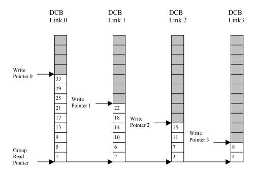
When links are deleted from a group, the DCB buffer depths of the remaining links are not effected. As shown in Figure 19, links 2 and 3 have been deleted from the group and the depth of the delay compensation buffers remain unchanged.
