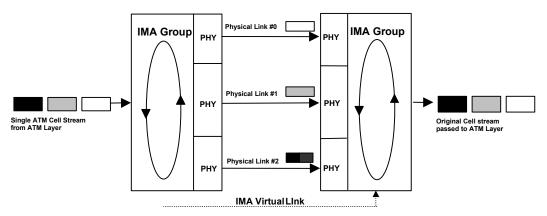
Tx direction cells distributed across links in round robin sequence Rx direction cells recombined into single ATM stream
