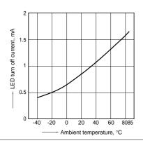
10. Off state leakage current
