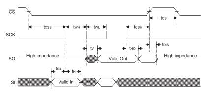
• Waveform 2 - Inactive clock polarity high
