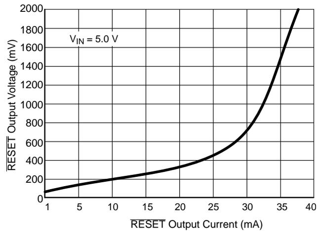
Figure 13.  $\overline{\text{RESET}}$  Output Voltage vs. Output Current
