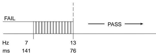
**Figure 20. WDI Signal for  $C_{Delay} = 0.82 \mu\text{F}$  using CS8141**
