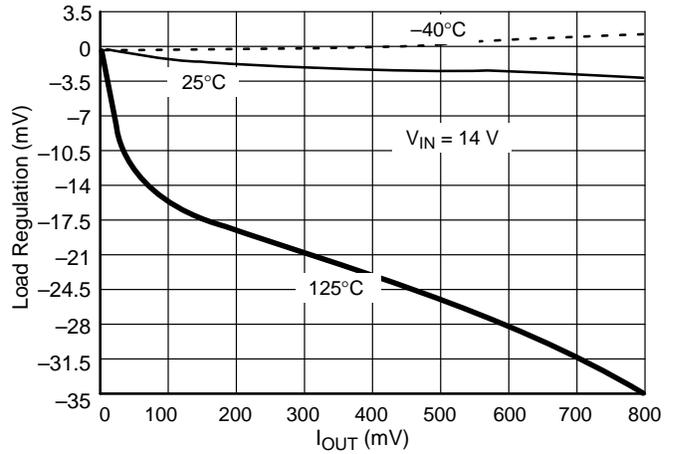
Figure 5. Load Regulation vs. Output Current Over Temperature
