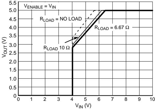
Figure 2.  $V_{OUT}$  vs.  $V_{IN}$  over  $R_{LOAD}$ ;  $T = 25^{\circ}\text{C}$
