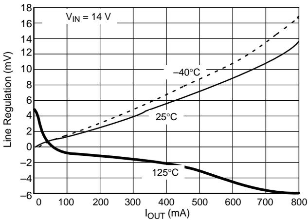
Figure 6. Line Regulation vs. Output Current Over Temperature
