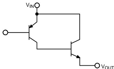
Figure 14. Composite Output Stage of the CS8140/1
