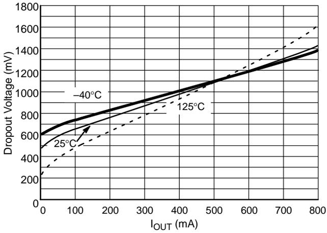
Figure 4. Dropout Voltage vs. Output Current Over Temperature
