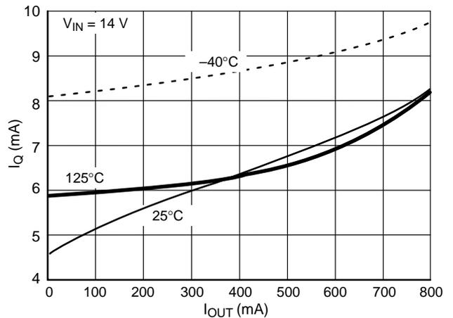
Figure 7. Quiescent Current vs. Output Current Over Temperature
