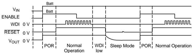
**WDI Frequency Rises Above the Upper Frequency Threshold After a Normal Period of Operation; ENABLE = LOW (for CS8140 only)**
