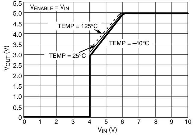
Figure 3.  $V_{OUT}$  vs.  $V_{IN}$  Over Temperature;  $R_{LOAD} = 25\ \Omega$
