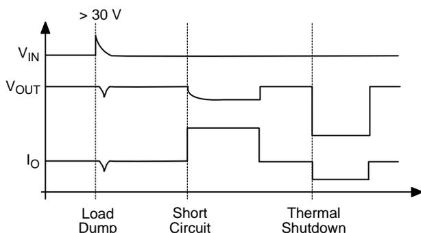
**Figure 15. Typical Circuit Waveforms for Output Stage Protection**
