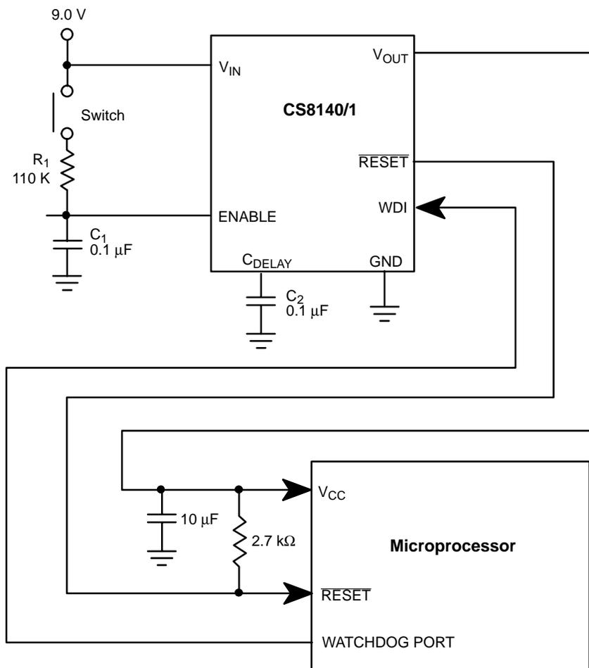
**Figure 21. Application Diagram for CS8140. The CS8140 Provides a 5.0 V Tightly Regulated Supply and Control Function to the Microprocessor. In this Application, the Microprocessor Controls its own Power Down Sequence (see text).**
