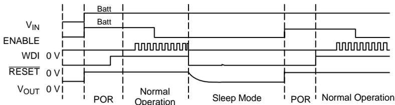
Figure 16. Timing Diagrams for Watchdog and ENABLE Functions
