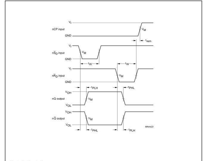
$V_{M}$  = 1.5 V at  $V_{CC} \geq 2.7$  V;
