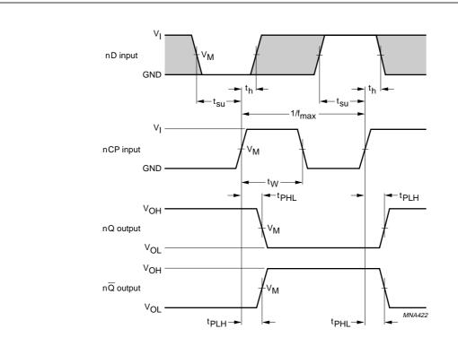
$V_{M}$  = 1.5 V at  $V_{CC} \geq$  2.7 V;
