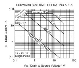
**Remark** Mounted on ceramic substrate of  $1200 \text{mm}^2 \times 0.7 \text{mm}$
