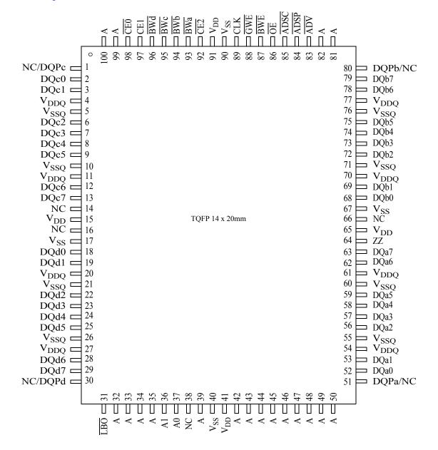
Note: For pins 1, 30, 51, and 80, NC applies to the x32 configuration. DQPn applies to the x36 configuration.
