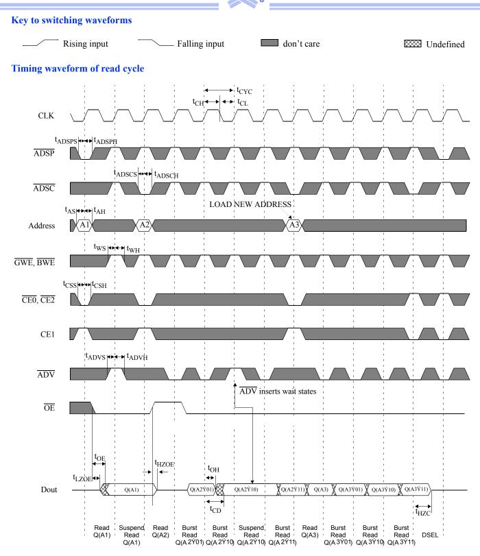
Note:  $\dot{Y} = XOR$  when  $\overline{LBO} = high/no$  connect;  $\dot{Y} = ADD$  when  $\overline{LBO} = low$ .  $\overline{BW[a:d]}$  is don't care.
