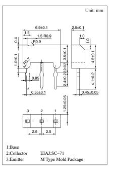
\* Printed circuit board: Copper foil area of 1cm<sup>2</sup> or more, and the board thickness of 1.7mm for the collector portion
