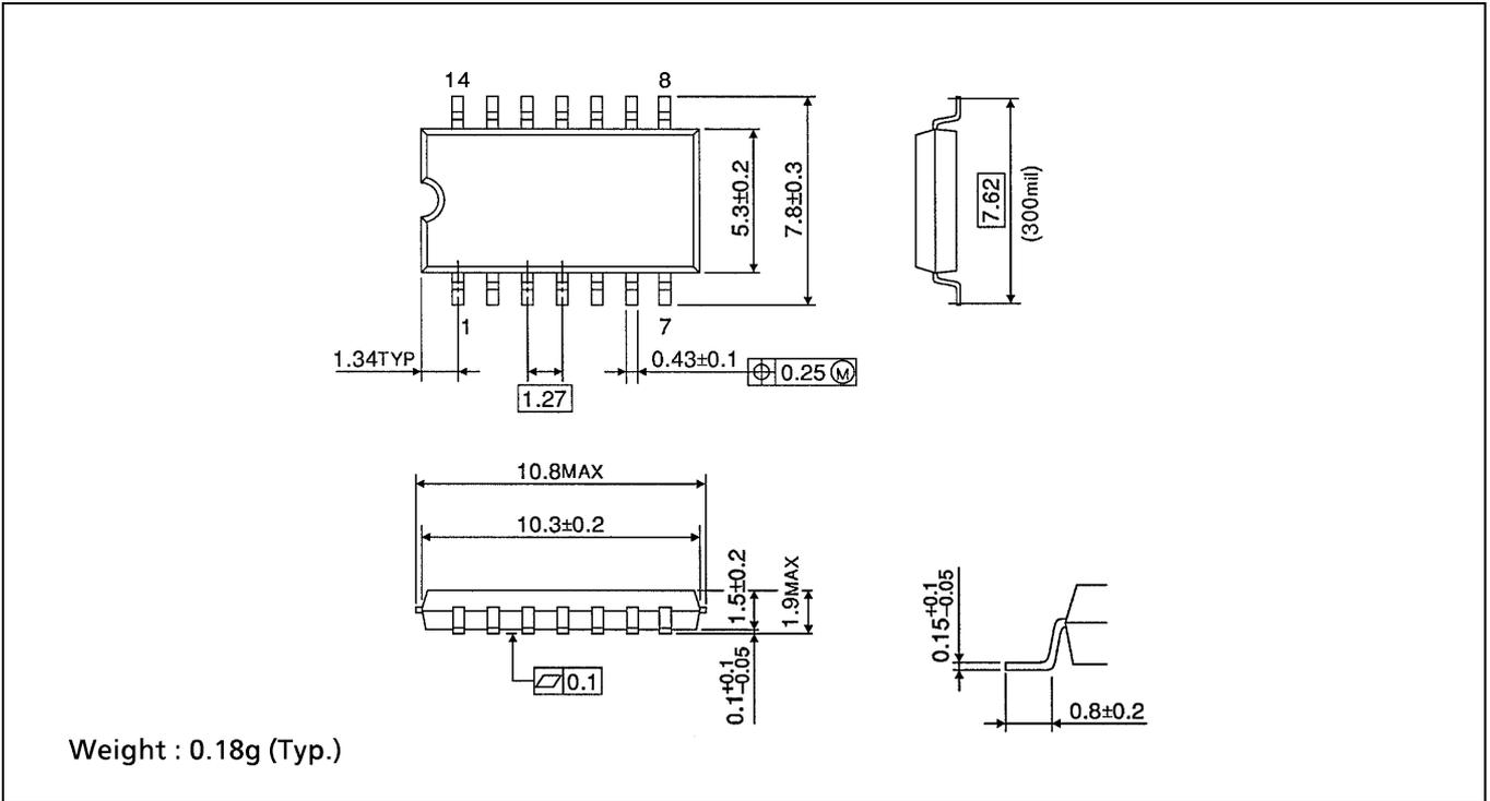
**SOP 14PIN (150mil BODY) PACKAGE DIMENSIONS (SOP14-P-150-1.27)**
