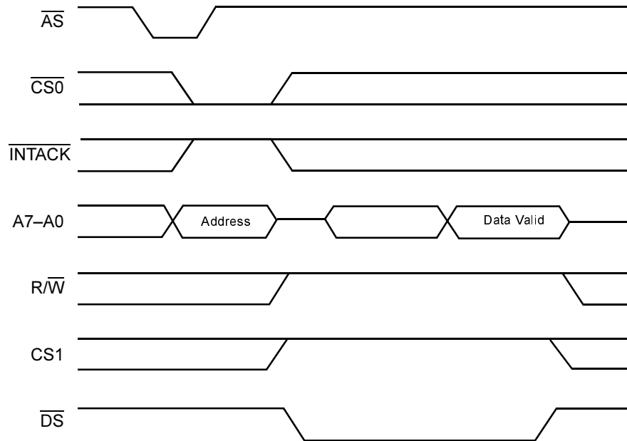
Figure 19. Z80230 Read Cycle Timing
