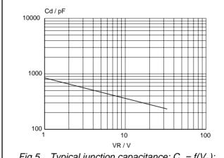
Typical junction capacitance;  $C_d = f(V_R)$ ; f = 1 MHz;  $T_j = 25^{\circ}\text{C}$  to  $125^{\circ}\text{C}$ .
