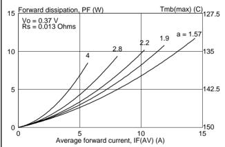
Fig.2. Maximum forward dissipation  $P_F = f(I_{F(AV)})$ ; sinusoidal current waveform where  $a = f(I_{F(AV)})$ ;  $factor = I_{F(RMS)} / I_{F(AV)}$ .
