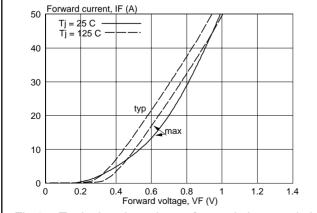
Fig.3. Typical and maximum forward characteristic  $I_F = f(V_F)$ ; parameter  $T_i$
