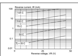
Fig.4. Typical reverse leakage current;  $I_R = f(V_R)$ ; parameter T<sub>i</sub>
