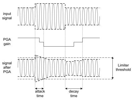
Figure 21 Limiter Operation
