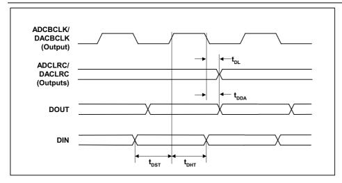
Figure 3 Digital Audio Data Timing – Master Mode
