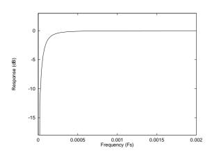
Figure 29 ADC Highpass Filter Response
