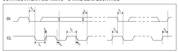
Figure 6 Control Interface Timing – 2-Wire Serial Control Mode (MODE=0)
