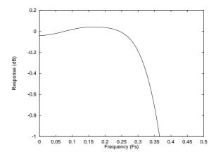
Figure 26 DAC Digital Filter Ripple (with DACOSR = 1) - 192kHz
