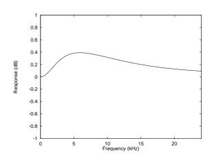
Figure 34 De-Emphasis Frequency Response (48kHz)
