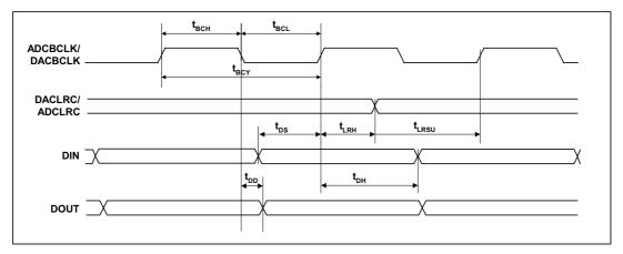
Figure 5 Digital Audio Data Timing - Slave Mode
