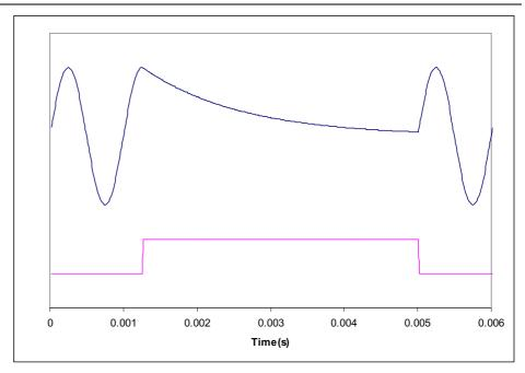
Figure 20 Application and Release of Soft Mute
