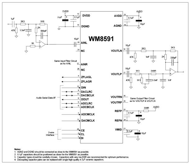
**Figure 36 Recommended External Components**
