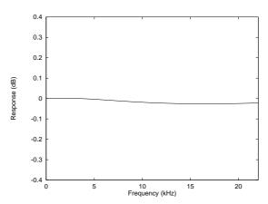
Figure 32 De-Emphasis Frequency Response (44.1KHz)
