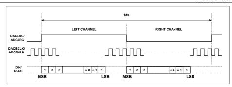
Figure 12 Left Justified Mode Timing Diagram
