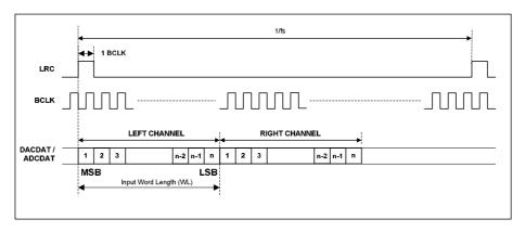
Figure 16 DSP/PCM Mode Audio Interface (mode B, LRP=1, Master)
