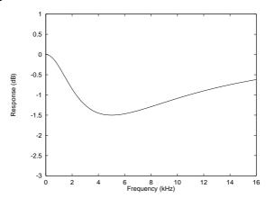
Figure 30 De-Emphasis Frequency Response (32kHz)
