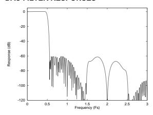
Figure 23 DAC Digital Filter Frequency Response -44.1, 48 and 96kHz
