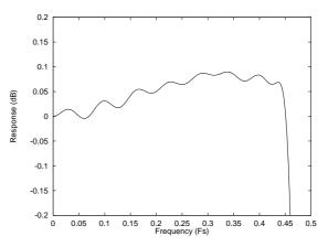
Figure 24 DAC Digital Filter Ripple -44.1, 48 and 96kHz
