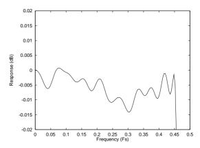
Figure 27 ADC Digital Filter Frequency Response
