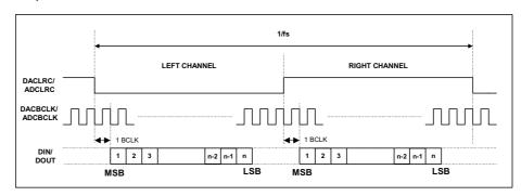
Figure 14 I<sup>2</sup>S Mode Timing Diagram
