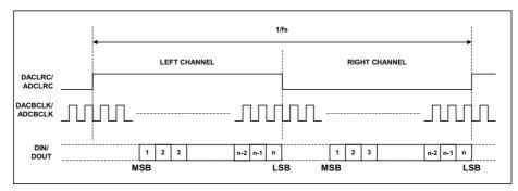
Figure 13 Right Justified Mode Timing Diagram
