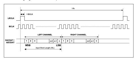
Figure 15 DSP/PCM Mode Audio Interface (mode A, LRP=0, Master)
