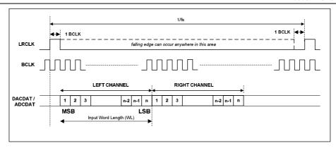
Figure 17 DSP/PCM Mode Audio Interface (mode A, LRP=0, Slave)
