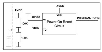
Figure 7 Internal Power on Reset Circuit Schematic
