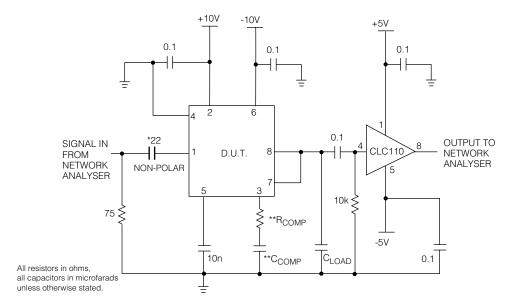
NOTES: This circuit can be used for Frequency Response, Delay and Differential Gain and Phase measurements.
