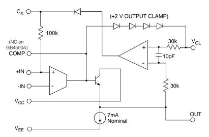
All resistors in ohms, all capacitors in microfarads unless otherwise stated
