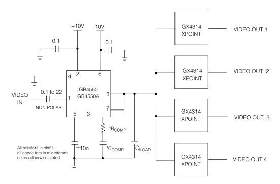
**NOTES**: In most applications  $R_{COMP}$  and  $C_{COMP}$  will not be needed since the bandwidth depends on the bus capacitance. In general, the maximum occurs when  $C_{LOAD}$  is between 82 pF and 100 pF.
