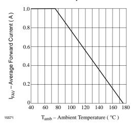
Figure 1. Max. Average Forward Current vs.
