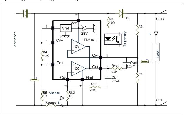
In the above application schematic, the TSM1011 is used on the secondary side of a flyback adapter (or battery charger) to provide an accurate control of voltage and current. The above feedback loop is made with an optocoupler.
