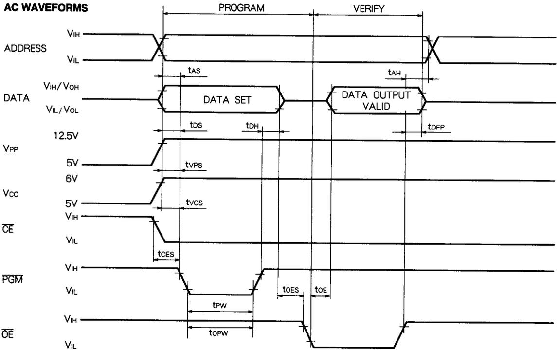
Test conditions for A.C. characteristics
