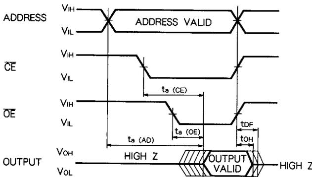
Test conditions for A.C. characteristics
